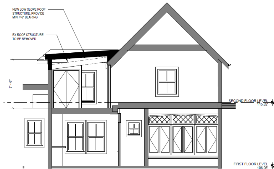
Figure 4 - Section showing proposed higher roof attached to existing gable and existing roof attachment.
