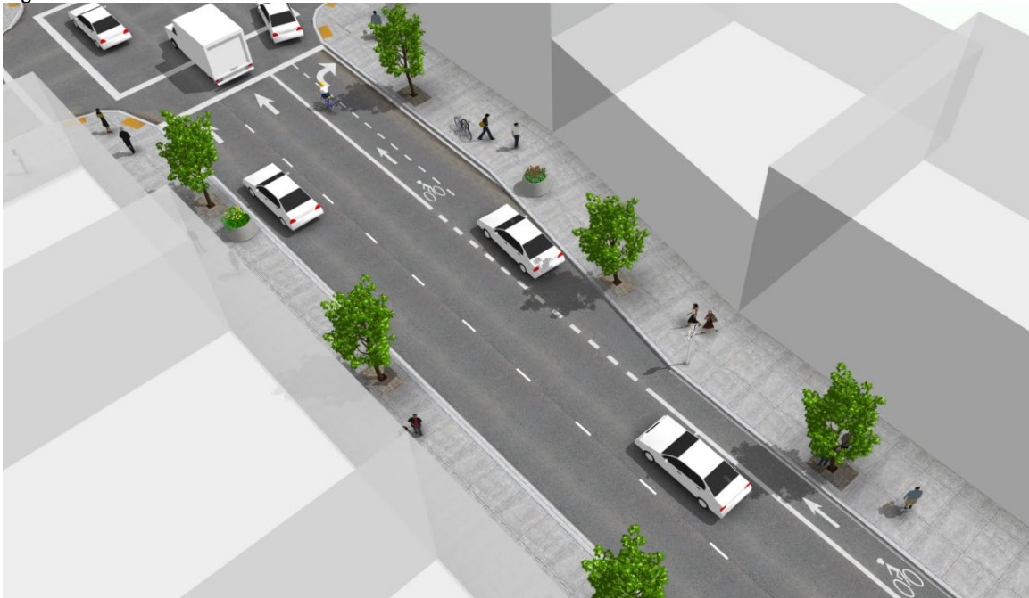
Figure 2-34. Combined Bike Lane/Turn Lane.
