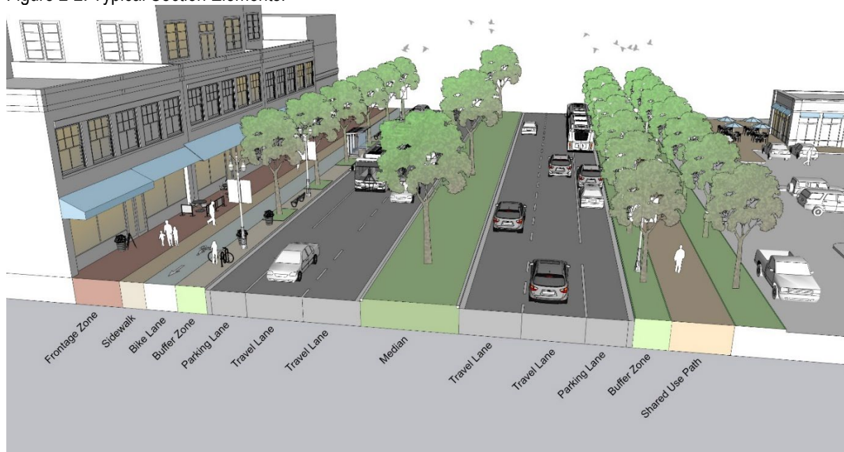
Figure 2-2. Typical Section Elements.
