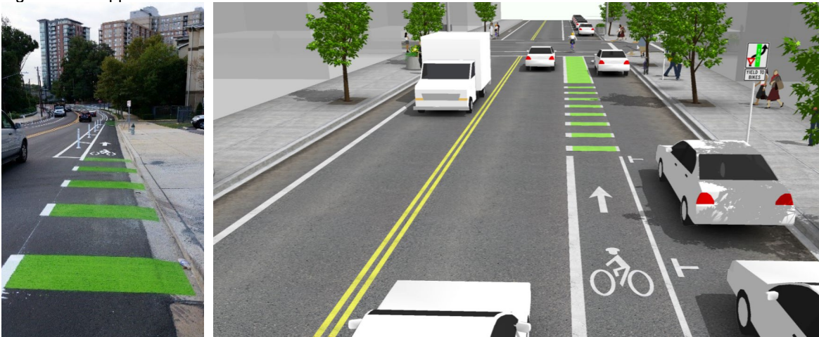
Figure 2-38. Application of Green Pavement Color in Conflict Zones.
