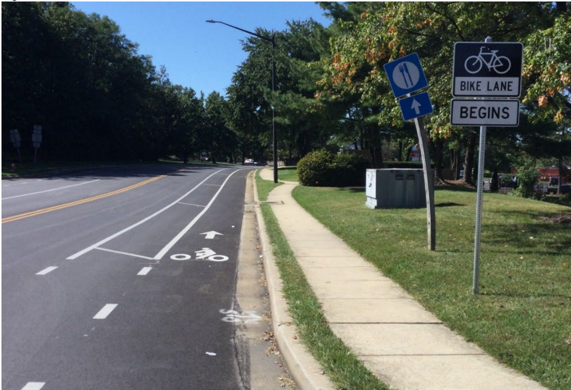
Figure 2-6. Buffered Bike Lane.
