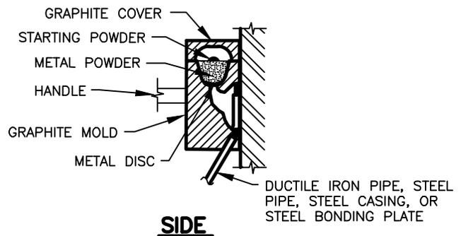
HOLD GRAPHITE MOLD FIRMLY OVER WIRE WITH OPENING AWAY FROM OPERATOR – IGNITE STARTING POWDER.
