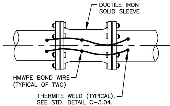
**TYPICAL BONDING OF SOLID SLEEVE**
