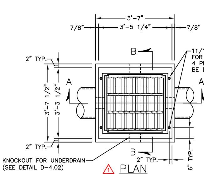
GALVANIZED 5/8" DIA. ANCHOR BOLT WITH DOUBLE NUT FOR ADJUSTING FRAME TO GRADE AND SLOPE. 4 BOLTS PER FRAME. LENGTH TO BE DETERMINED IN THE FIELD.
