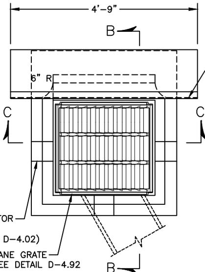
KNOCKOUT FOR UNDERDRAIN (SEE DETAIL D-4.02)
