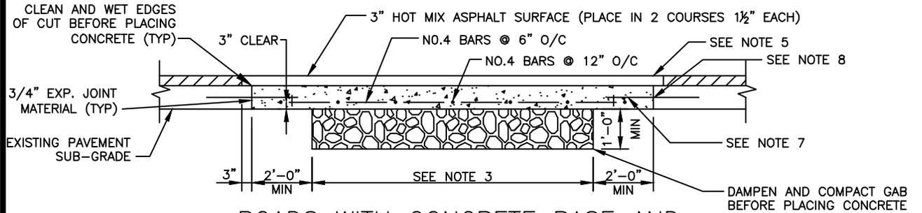
**ROADS WITH CONCRETE BASE AND HOT MIX ASPHALT SURFACE**
