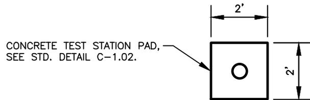
CONCRETE TEST STATION PAD,
