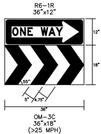
\* NOTE: MUST BE FABRICATED AS ONE SIGN (ONE PIECE OF SHEET ALUMINUM)
