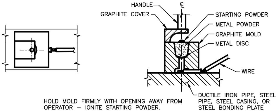
HOLD MOLD FIRMLY WITH OPENING AWAY FROM OPERATOR - IGNITE STARTING POWDER.
