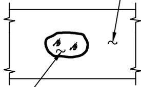
CLEAN SURFACE TO BRIGHT METAL AT WELD LOCATION WITH MECHANICAL GRINDER.
