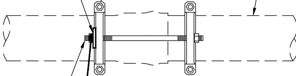
ATTACH CONNECTOR PLATE TO RESTRAINING HARNESS AT TIE BOLT, SEE NOTE 3.
