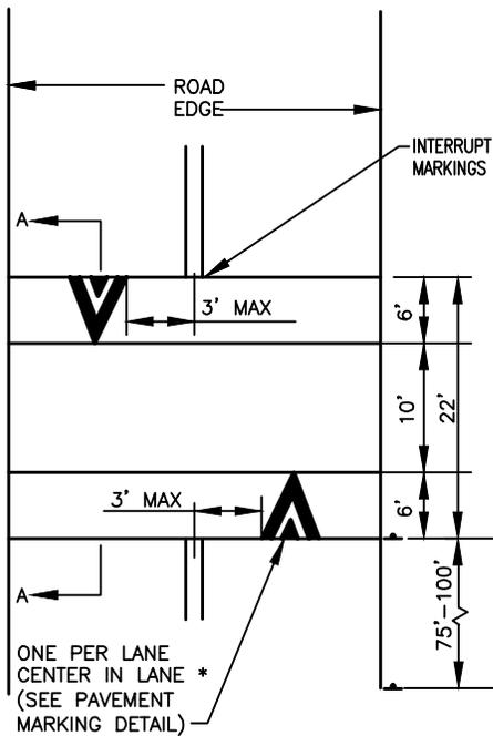
\* WHEN NO CENTERLINE PRESENT, CONTACT COUNTY TRAFFIC DIVISION FOR PROPER LOCATION OF PAVEMENT MARKING
