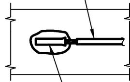
STRIP INSULATION FROM WIRE. INSTALL SLEEVE ON WIRE.
