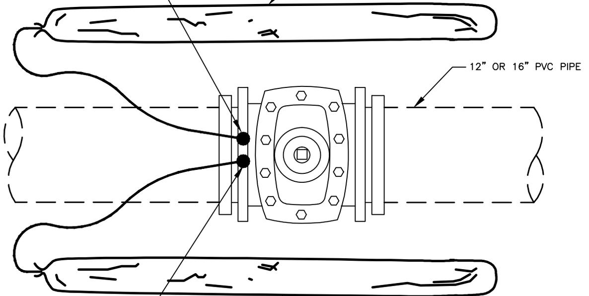
THERMITE WELD ANODE LEAD WIRE DIRECTLY TO DUCTILE IRON VALVE, SEE STD. DETAIL C-3.04.
