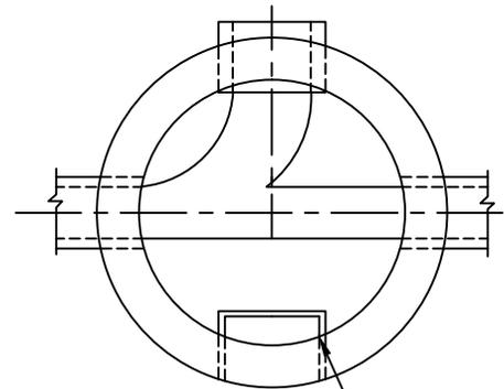
MANHOLE STEPS SHALL BE INSTALLED PARALLEL TO BENCH, AWAY FROM PIPE OPENINGS
