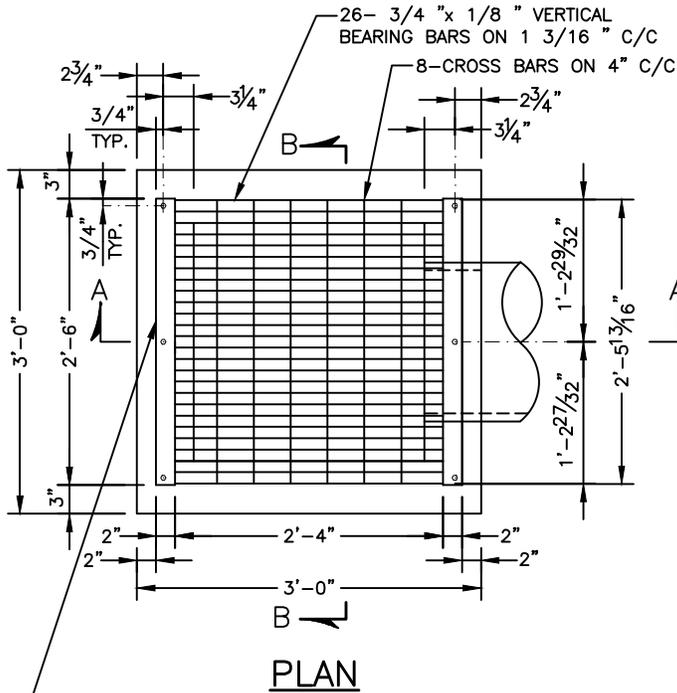
2- 2"x 1 1/4 "x 3/16 "x2'-6" (CENTERED ON GRATE) TRIM VERTICAL LEG OF ANGLE TO 3/4 " IN HEIGHT WELD SECURELY TO GRATING AT EVERY 4TH BAR (WELDED AREAS TO BE TOUCHED UP WITH ZINC RICH PAINT AFTER WELDING.)
