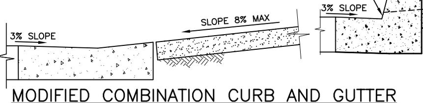
**MODIFIED COMBINATION CURB AND GUTTER**
