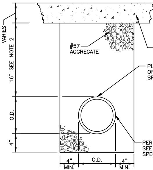
**PAVEMENT SUB-BASE UNDERDRAIN
