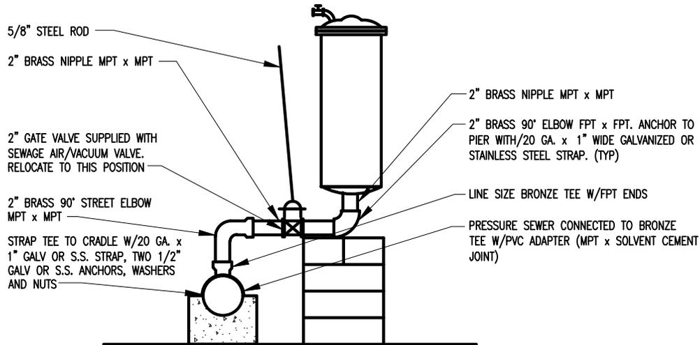
**CONNECTION AIR/VACUUM VALVE TO MAINLINE PRESSURE SEWER**
