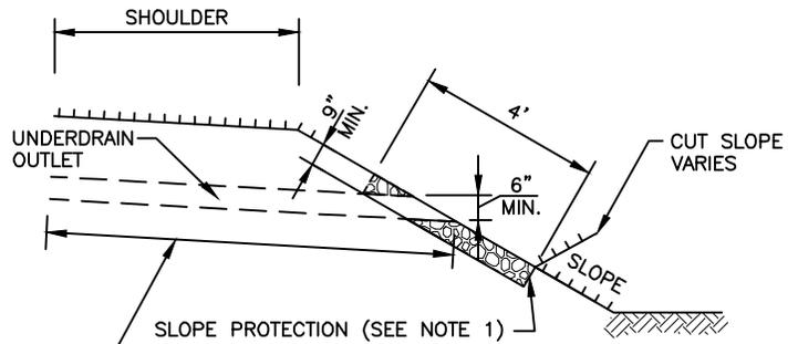
THIS 10' SECTION SHALL BE CIRCULAR, CORRUGATED METAL PIPE OF THE SIZE INDICATED ON THE PLANS REGARDLESS OF THE TYPE OF PIPE USED FOR THE REMAINDER OF THE SUB-SURFACE DRAINAGE SYSTEM
