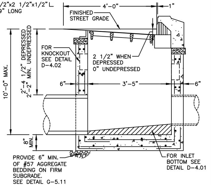
PROVIDE 6" MIN. OF #57 AGGREGATE BEDDING ON FIRM SUBGRADE. SEE DETAIL G-5.11
