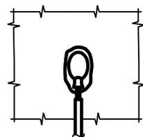
REMOVE SLAG FROM CONNECTION. THOROUGHLY CLEAN WELD AREA.
