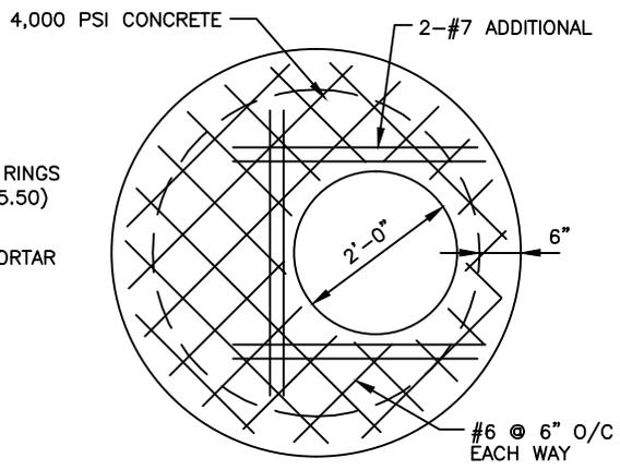
**SLAB REINFORCING SHALLOW PRECAST MANHOLE**
